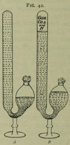
Fermentation tubes, showing method of testing gas-producing power. A, growth of a non-gas-producer; B, growth of a gas-producer
