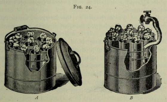
Apparatus for home pasteurization, arranged for heating, and also as connected with water faucet for cooling.
