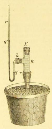
Fig. 1150. Apparatus for the estimation of root-pressure. (After Sachs.)
