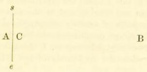
Thus, let se (fig. 2) be a vertical section of the screen. When the reed was at A and the flame at B there was no action; when the reed was at B and the flame at A the action was decided. It may be added that the vibrations communicated to the screen itself, and from it to the air beyond it, were without effect; for when the reed, which at B was effectual, was shifted to C, where its action on the screen was greatly augmented, it ceased to have any action on the flame at A.
