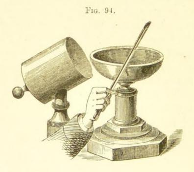
brought near the vibrating bell, the resonance is feeble. On lengthening the tube by drawing out the slider, at a certain point the tone swells out as before. If the tube be made longer, the resonance is again enfeebled. Note the fact, which shall be explained presently, that the open tube which gives the maximum resonance is exactly twice the length of the closed one. For these fine experiments we are indebted to Savart.
