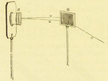
(B is the bi-refracting spar, dividing the incident light into the two beams o and e; G is the mirror.) The beam is here reflected *laterally*. When the reflection is upwards, the other beam is reflected as shown in fig. 33.
