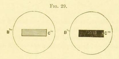
Let us push our test still further. By means of an endless screw, the crystal can be turned ninety degrees round. The black image, as I turn, becomes gradually brighter, and the bright one gradually darker; at an angle of forty-five degrees both images are equally
