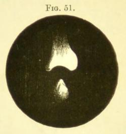
ray-filter, and placing at the focus a thin sheet of platinized platinum, the invisible rays declare their presence and distribution by stamping upon the platinum a white-hot image of the carbons. (See fig. 51.)
