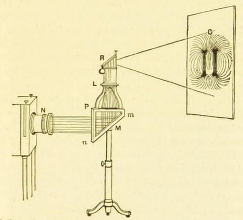
N is the nozzle of the lamp; M a plane mirror, reflecting the beam upwards. At P the magnets and iron filings are placed; L is a lens which forms an image of the magnets and filings; and R is a totally-reflecting prism, which casts the image G upon the screen.
