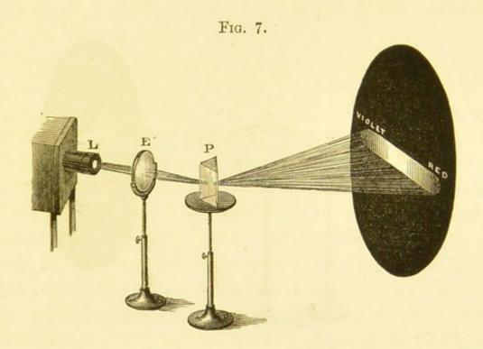
(from L, fig. 7) which produces the disk to pass through a lens (E), which forms an image of the aperture, and then through a prism (P), we obtain Newton's coloured image, with its red and violet ends, which he called *a spectrum*. Newton divided the spectrum into seven parts—red, orange, yellow, green, blue, indigo, violet; which are commonly called the seven primary or prismatic colours. The drawing out of the white light into its constituent colours is called *dispersion*.
