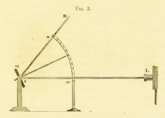
suffices to show the equality; while if the graduated arc of the angles be consulted, the arc from 5 to m is found accurately equal to the arc from 5 to n. The complete expression of the law of reflection is not only that the angles of incidence and reflection are equal, but that the incident and reflected rays always lie in a plane perpendicular to the reflecting surface.
