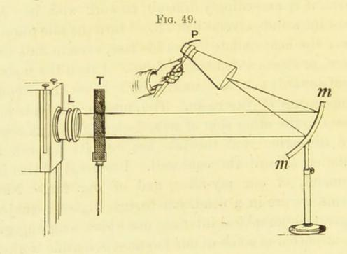
pile the positions of the invisible reflected beam, we prove that the angular velocity of the heat-beam, like that of the light-beam, is twice that of the mirror.
