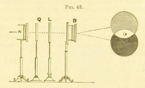
colours are superposed we have a pure white. (See fig. 43, where N is the end of the polarizer, Q the quartz plate, L a lens, and B the bi-refracting spar. The two images overlap at O, and produce white by their mixture.)
