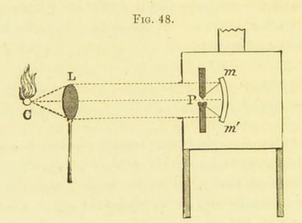
and placed behind the carbons (P). By this mirror we can cause the rays to issue through the orifice in front of the camera, either parallel or convergent. They are now parallel, and therefore, to a certain extent, diffused. We place a convex lens (L) in the path of the beam; the light is converged to a focus (C), and at that focus paper is not only pierced, but it is instantly set ablaze.
