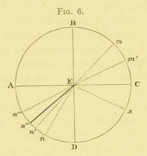
water all, but will be *totally* reflected (along E x). At the under surface of the water, moreover, the law is just the same as at its upper surface, the angle of incidence (D E n''') being equal to the angle of reflection (D E x).
