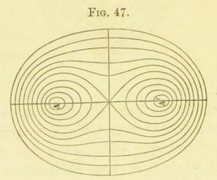
of these crystals, suitably cut, are placed between the polarizer and analyzer, the axes (A A', fig. 47) are seen surrounded, not by circles, but by curves of another order and of a perfectly definite mathematical character. Each band, as proved experimentally by Herschel,
