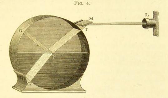
O) is rendered clearly visible. It is also seen that *reflection* (along O R) accompanies refraction, the beam dividing itself at the point of incidence into a refracted and a reflected portion.<sup>1</sup>
