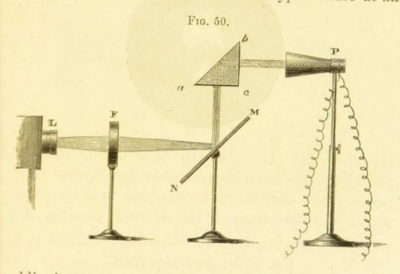
obliquity greater than the limiting angle,<sup>1</sup> and 1s therefore totally reflected. Quenching the light by the ray-filter at F, and placing the pile at P, the totallyreflected heat-beam is immediately felt by the pile, and declared by the galvanometric deflection.
