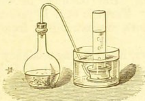
FIG. 16.—Apparatus for watching Alcoholic Fermentation.
