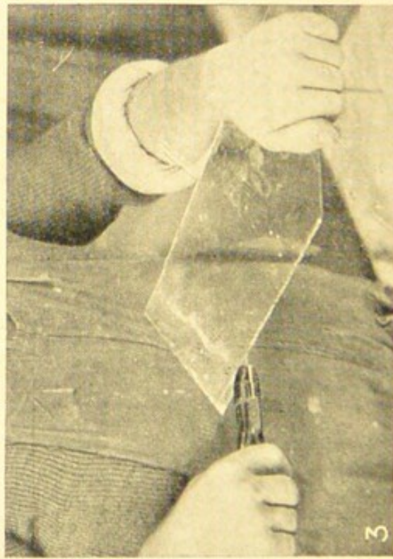
GLASS CUTTING. Fig. 1. How to hold the diamond. Fig. 2. Bench arrangement of battens and pliers. Fig. 3. Breaking away the glass with pliers. Fig. 4. How to cut a hollow, curved piece of glass. Note criss-cross cuts and use of diamond to tap out the pieces.
