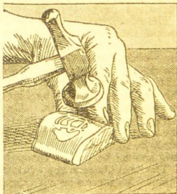
PIERCED METAL WORK. Fig. 2, Above. How saw and table are used. Fig. 3, Right. Shaping ring on a wooden block
