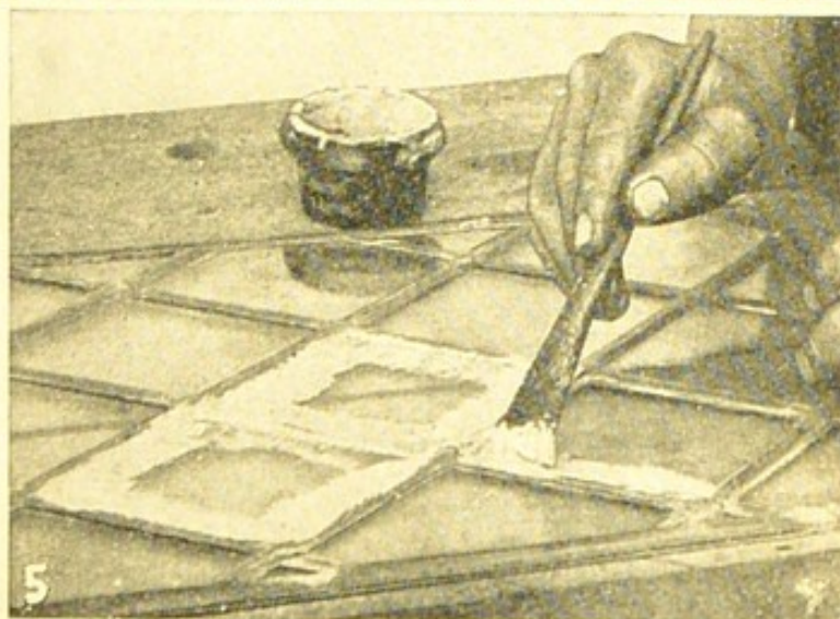
Fig. 1. First steps. Fig. 2. Three pieces of glass in place, the calms held by pins. Fig. 3. Soldering the joints. Fig. 4. Turning panel over to solder other side. Fig. 5. Brushing cement into joints
