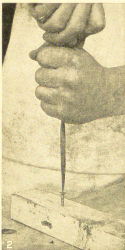
Left. Showing double-handed grip necessary for a large screwdriver. Right. Using screwdriver bit in brace
