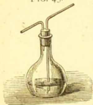
The ammonium sulphide is contained in a small wash bottle, the exit-tube of which is cut short so as not to dip into the liquid, while the blowing tube passes nearly to the bottom of the flask. (See fig. 45.)
