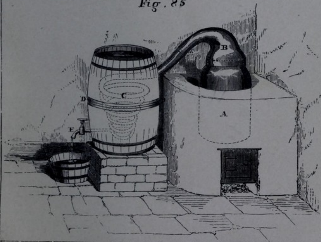
Fig. 84.—APPARATUS FOR VINEGAR MAKING BY THE QUICK PROCESS. „ 85.—SMALL STILL.
