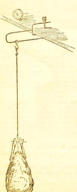
This represents a model of a Chimney Screw-jack for suspending joints to. Its cost is very trifling, and may be purchased at any ironmonger's. It will fit on any mantel-shelf; and it enables the joint to be shifted nearer or further from the fire, as occasion requires.
