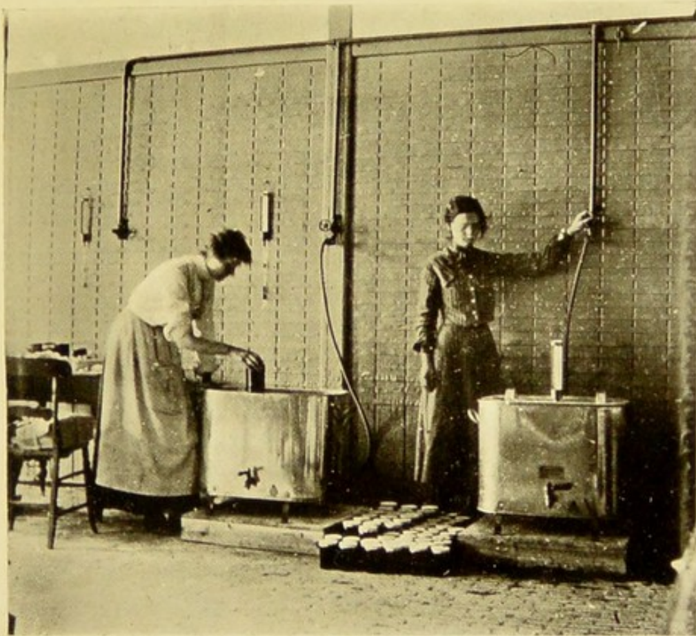
MERCIA PATENT STERILISER. SIZE A. HEAT SUPPLIED BY STEAM. VALVE OF STEAM JET, BEING TURNED ON BY OPERATOR
