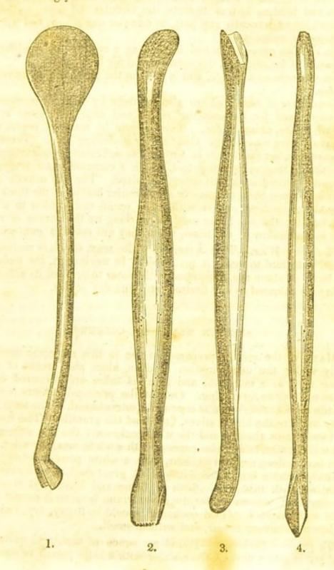
Modelling Tools.—No. I is termed the rose-stick, the thin flat end being used for forming the leaves of roses out of modelling wax by flattening a piece of it on a table until it is of the required form and size; the other end is used for fluting and making borders.
