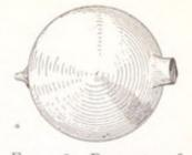
FIG. 126.— Resonator of von Helmholtz.
