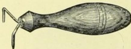
Handle for Lifting the Blowpipe Pad. The points can be inserted in any two of the loops on the metal band, which is fixed round the asbestos.
