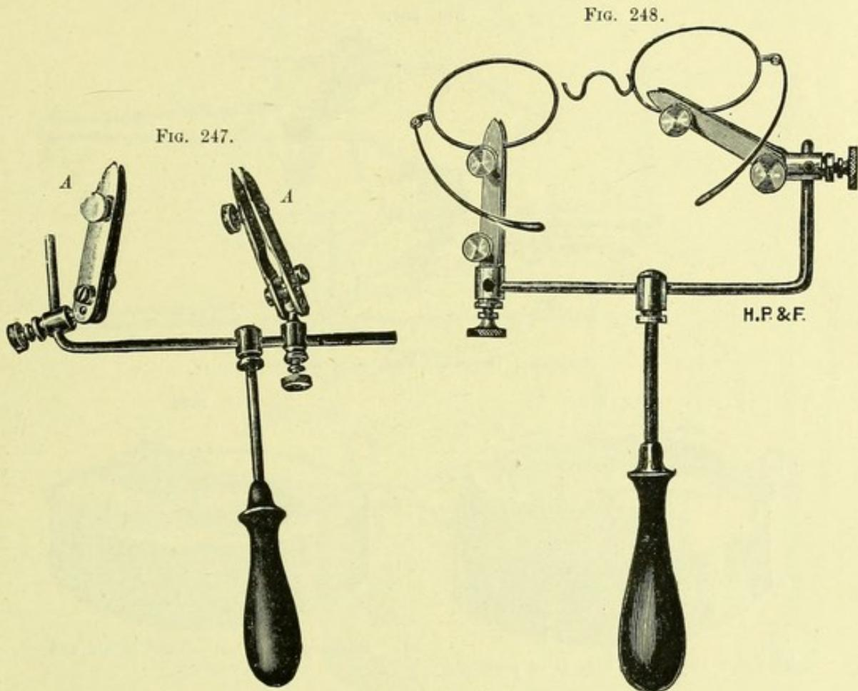
Fig. 247.—SOLDERING GRIP for holding articles in any position. A small object can be conveniently secured between the jaws *A A* when they are set near enough to each other.
