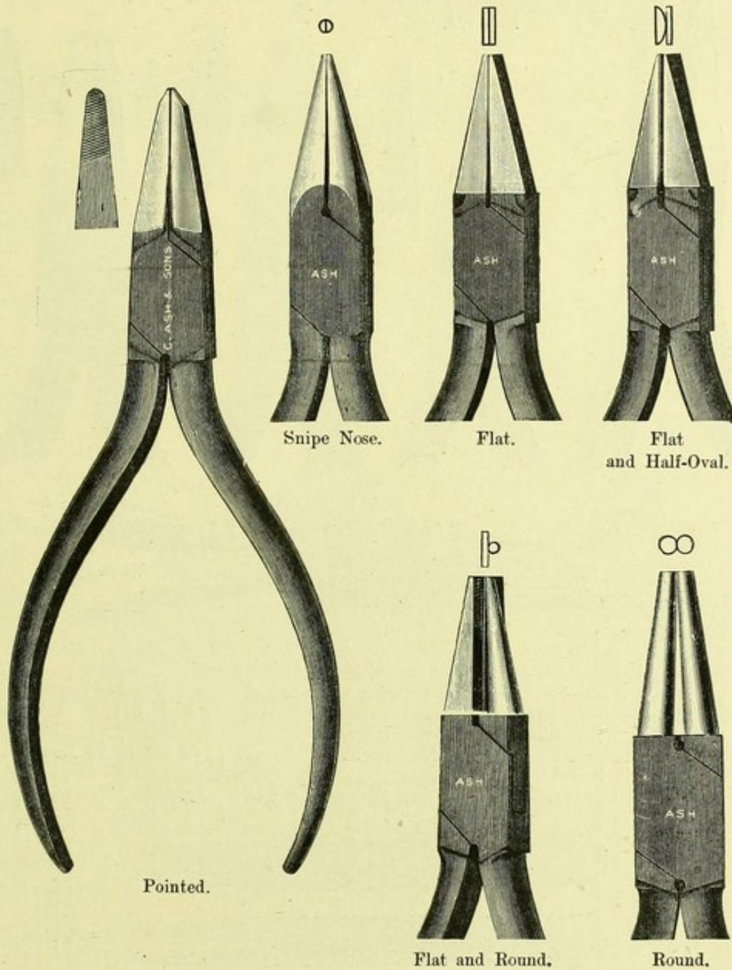
Of these Pliers, the two sizes most generally used are the  $4\frac{1}{2}$  and 5 inch lengths.
