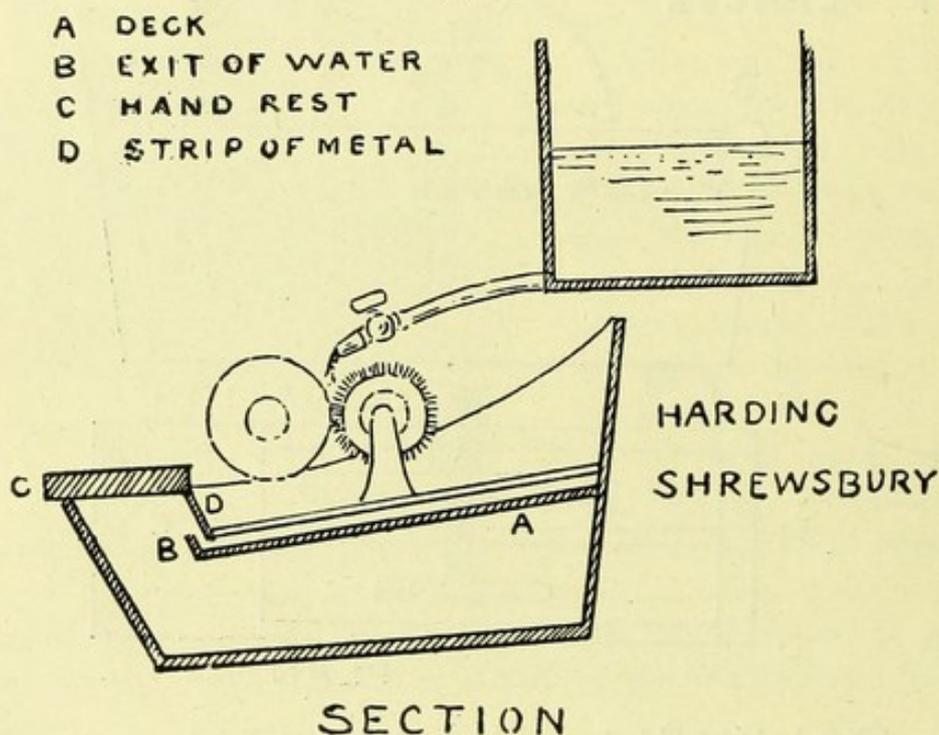
GRINDING LATHE HEAD, ETC.
