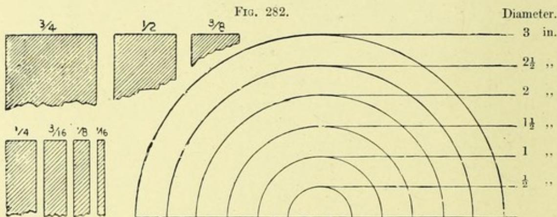
CARBORUNDUM LATHE WHEELS (Sizes and Thicknesses.)
