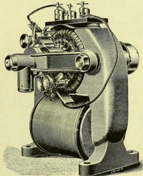
CUTTRISS, WALLIS &amp; Co.'s "RING" MOTOR (R/3). half-horse power, suitable for driving two or three workroom lathes.
