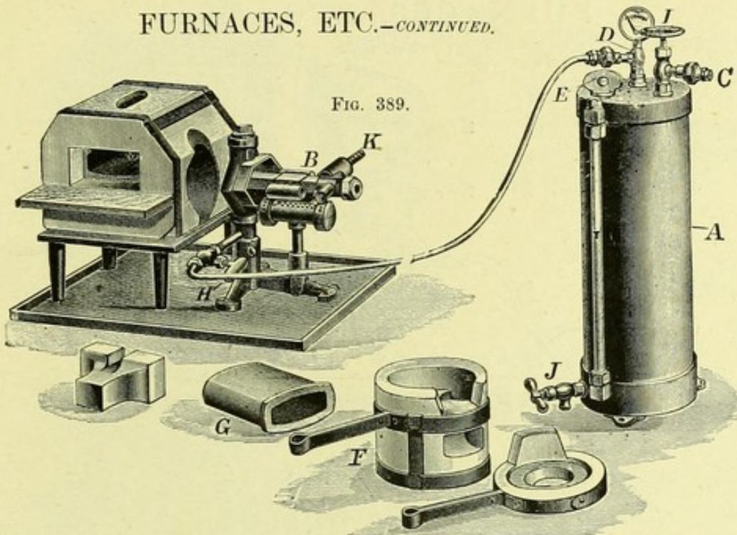
MR. GARTRELL'S CONTINUOUS-GUM FURNACE, ETC., WITH PETROLEUM BLAST.
