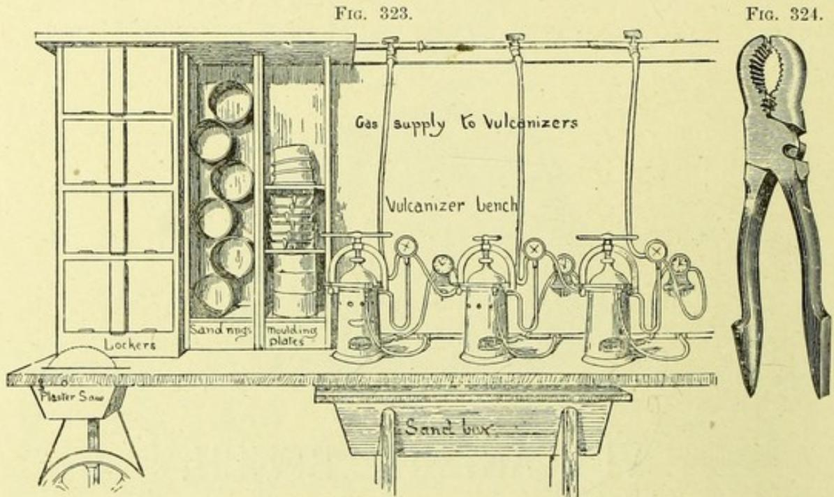
Fig. 323.—AUTHOR'S VULCANIZER BENCH, showing:—(a) Plaster Saw; (b) Lockers; (c) Sand Rings; (d) Moulding Plates; (e) Sand Box; (f) Gas Supply and Taps; also Vulcanizers, the Stands of which are screwed to Bench, and Compo Pipe leading to external air, connected with Screw Taps for blowing off steam from the Vulcanizer boilers.
