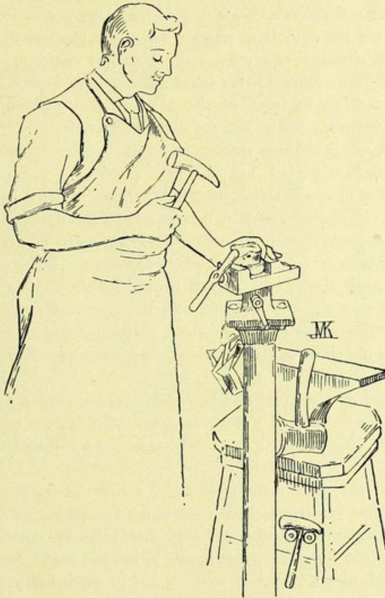
DRILLING MACHINE VICE ON IRON PILLAR HOLDING DIE IN POSITION FOR USE OF HORN MALLET.
