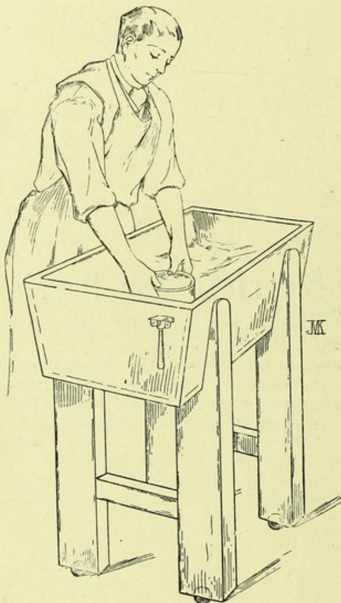
AUTHOR'S SAND-MOULDING TROUGH, with shelf in it for moulding on.
