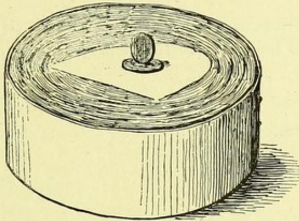
MOULDING RING WITH MR. LENNOX'S LIFTER ATTACHED TO PLASTER MODEL.
