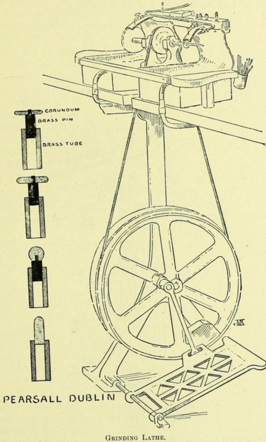
I regard the use of a strip of leather in this way by Mr. Biggs as a very great advance on the methods commonly used. This grinding lathe is run by a fly wheel attached to the floor.
