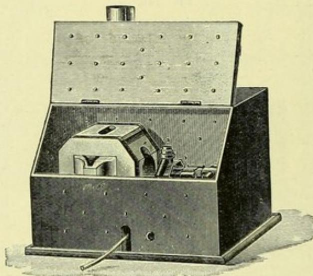
HOOD MADE OF SHEET-IRON, LINED WITH ASBESTOS, FOR PLACING OVER THE FURNACE TO MUFFLE THE NOISE.
