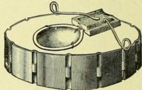
Blowpipe Pad, with Ingot Mould and Crucible.
