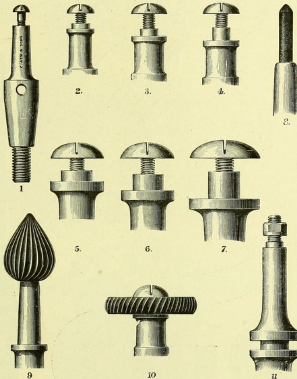
CHUCKS FOR LATHE HEAD, Fig. 281.
