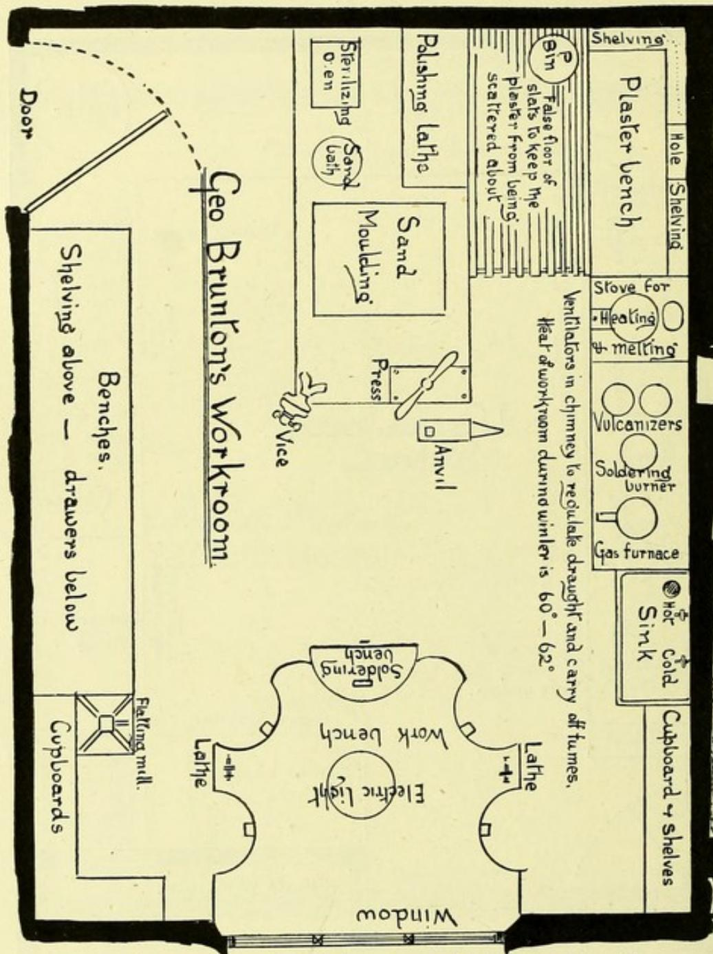
Electric light from roof. can be pulled down and shifted where required
