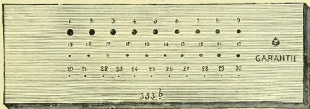
DRAWPLATE, with 30 holes for round wire. (Drawplates with half-round and with square holes are also very useful.)
