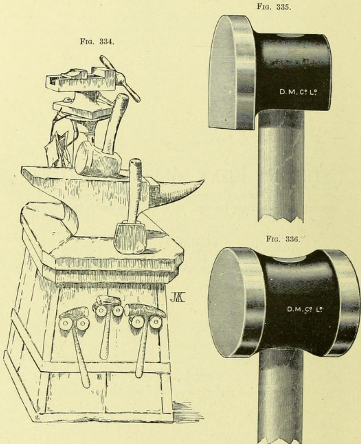
Fig. 334.—AUTHOR'S STRIKING BLOCK, with Smith's Anvil, Striking Hammers, Horn Mallets and Drilling Machine Vice—see also Fig. 54, page 91.
