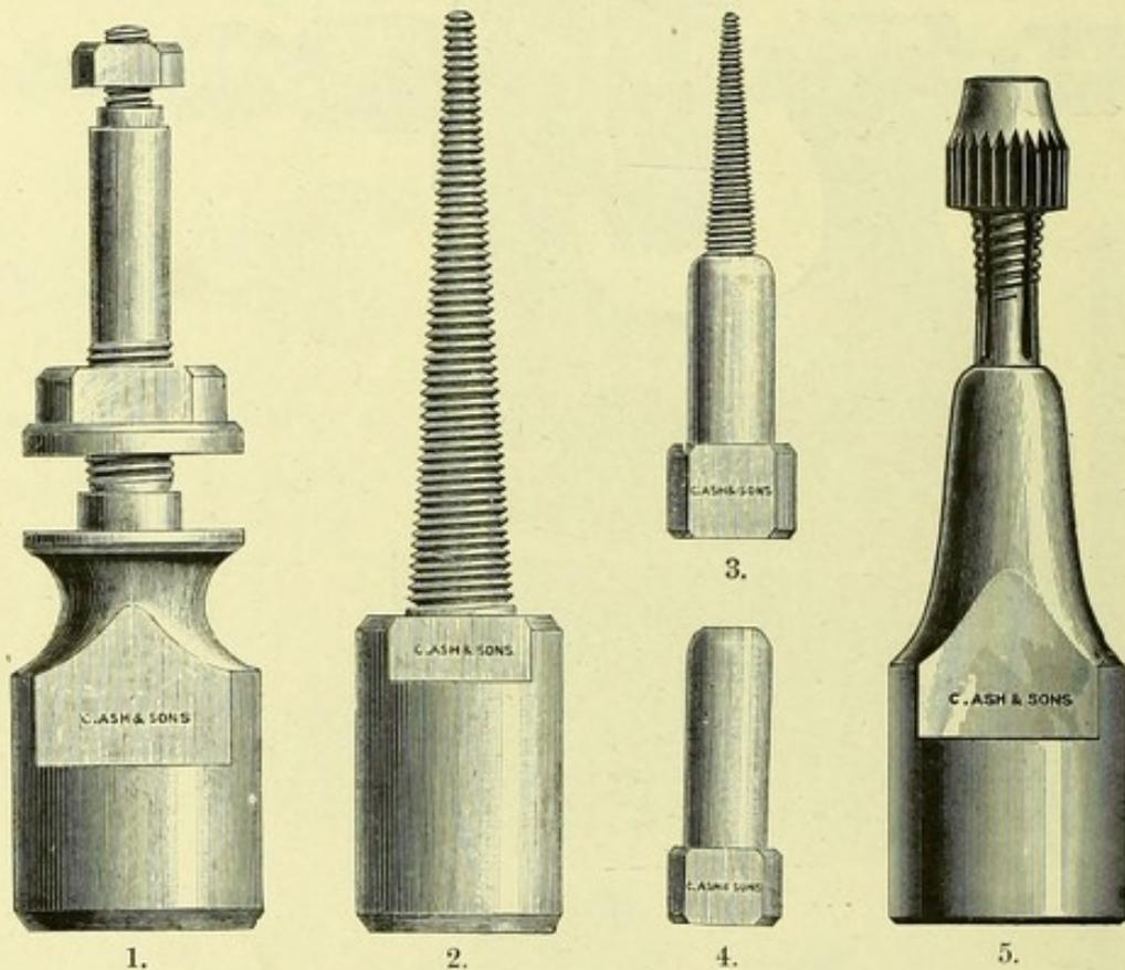
CHUCKS FOR LATHE HEADS, Figs. 286, 287.
