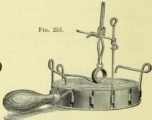
Blowpipe Pad, showing vertical and horizontal wires which support the clamp that holds a band while it is being soldered.
