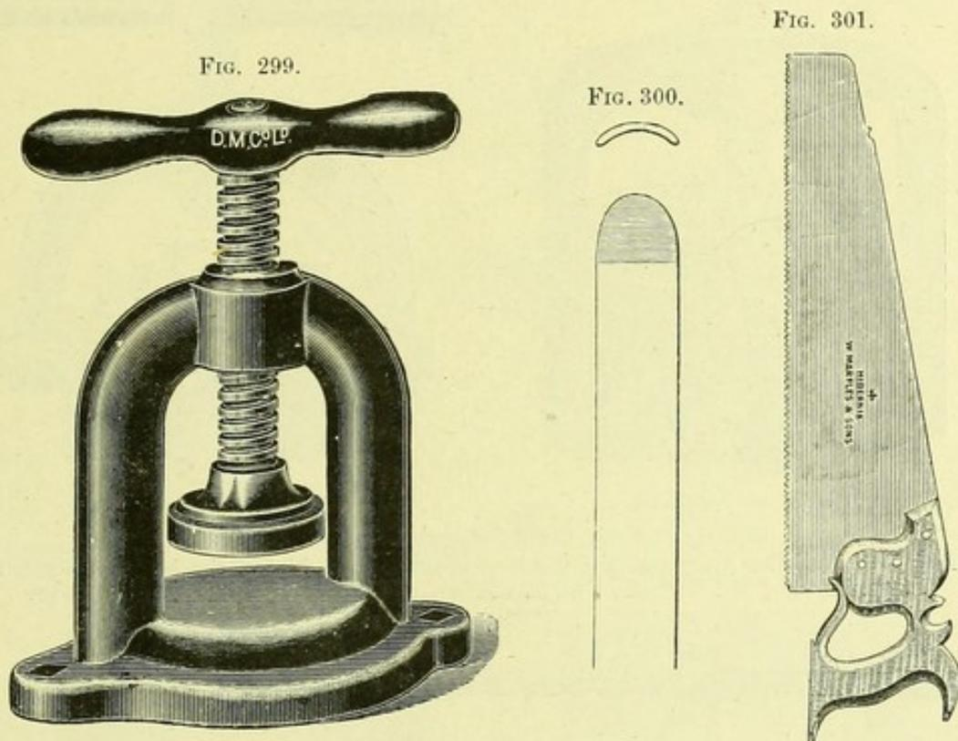
Fig. 299.—SCREW PRESS for closing Vulcanite Flasks.
