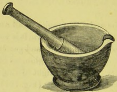
Fig. 101 shows a pestle and mortar for breaking up the copper amalgam when heated. For this purpose they should be constructed of either agate or glass, as the compound adheres to Wedgwood's composition.
