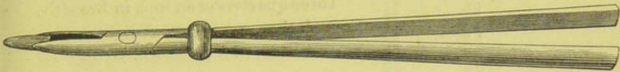
Fig. 123 shows a steel holder for carrying arkansas or corundum points for polishing stoppings.
