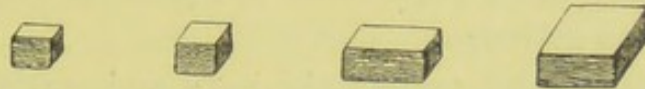
Fig. 128 shows the form in which gold foil prepared in blocks with parallel layers is now vended.
