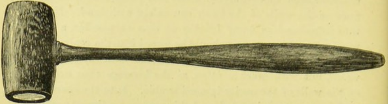
Fig. 116 shows a hand mallet, the head of which is constructed of hard wood filled with lead, which lessens the amount of vibration when used.
