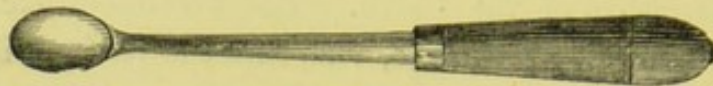
Fig. 100 shows an iron spoon or ladle with wooden handle for heating, over a spirit-lamp, the copper (Sullivan's) amalgam.
