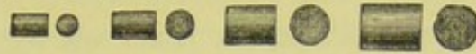
Fig. 127 shows the form in which gold foil prepared in cylinders is now vended.
