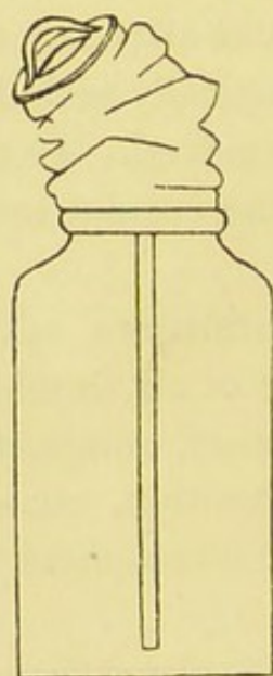
FIG. 38.—The flexible bellows-pump employed by Angus Smith to draw out air from the air jar.
