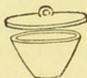
FIG. 6.—Crucible with lid.
