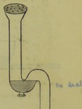
Fig. 81.—Siphon Sink Trap, with movable screw for cleaning.
