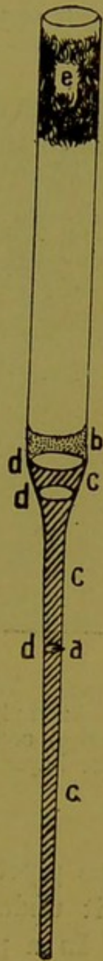
FIG. 18.—Showing method of filling pipette. a. Is the mark on the tube. b. The serum. c, c, c. The columns of emulsion separated by the air bubbles d, d, d. e. Is the cotton-wool plug.
