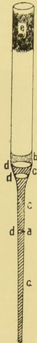
FIG. 24.—SHOWING METHOD OF FILLING PIPETTE.
