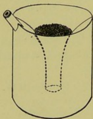
Fig. 88. — Counterpoise; weight when empty, 35 grammes; when full of dust shot, 200 grammes.
