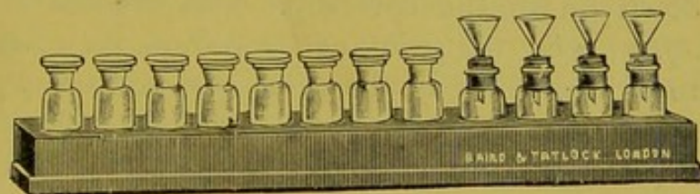
FIG. 12.—STAND FOR STAINING REAGENTS Four of the bottles are fitted with glass filters passing through rubber stoppers.
