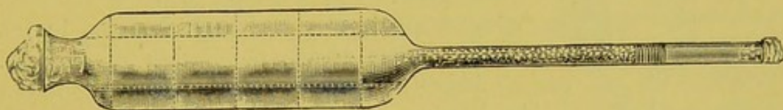
FIG. 131.—AËROBIOSCOPE EMPLOYED IN THE METHOD OF SEDGWICK AND TUCKER, FOR THE BACTERIOLOGICAL ANALYSIS OF AIR
