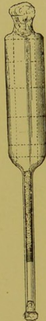
FIG. 39.—Sedgwick's expanded tube for air-examination.
