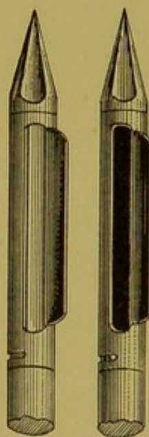
FIG. 43.—Fränkel's instrument for obtaining earth from various depths for bacteriologic study.
