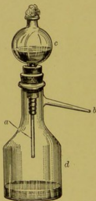
FIG. 13.—Kitasato's filter: a , porcelain bougie; b , attachment for suction-pump; c , reservoir; d , sterile receiver.
