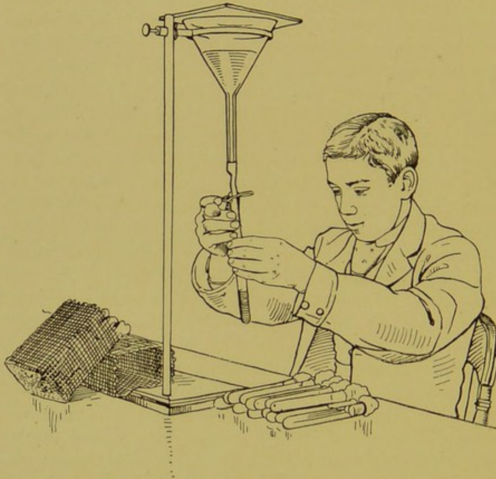
FIG. 17.—Funnel for filling tubes with culture-media (Warren).
