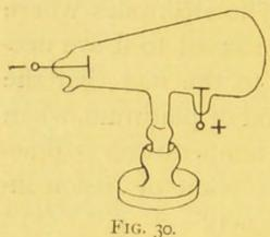
Crookes tube having two electrode disks of aluminum, the one in the end to be used as the cathode and the lower one the anode.
