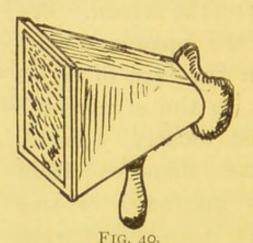
like the heart, liver and spleen, may be outlined. Of this more will be said in detail later on. A sketch of the Edison fluoroscope is shown in Fig. 40. This instrument is manufactured by Messrs. Aylesworth &
