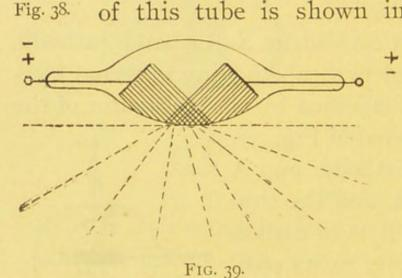
two slanting plate or disk electrodes mutually converge the cathodic stream to a concentrated area of
