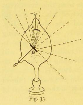
be used as the anode. This is essentially the focus or reflector type of tube which has superseded the globular and pear-shaped tubes and which is now generally in use. The only essential difference is that the anode B may be bent one way or the other to a greater or less extent.
