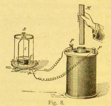
the coil back and forth we get similar results to those in section 4. That is, when we move the coil towards the magnet we induce a momentary current in one direction and when we
