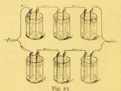
times the voltage and twice the ampèrage of a single unit.
