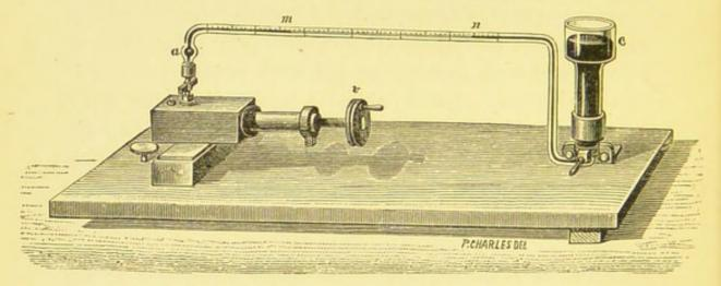
FIG. 8.—Apparatus of Bonnier and Mangin, for analysis of gases given off by plants. c, *Reservoir of Mercury*; *m m*, graduated tube; *v*, screw of piston, which enables the gas to be drawn into the graduated tube and measured; and after it the potash and pyrogallic solutions successively each being thoroughly brought into contact with the gas in the dilatations *a*.
