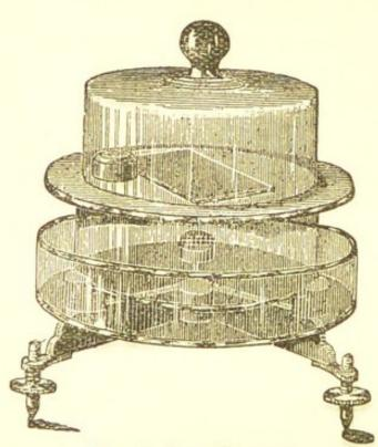
Fig. 22. Damp Chamber. (For plate-cultivation, etc.)
