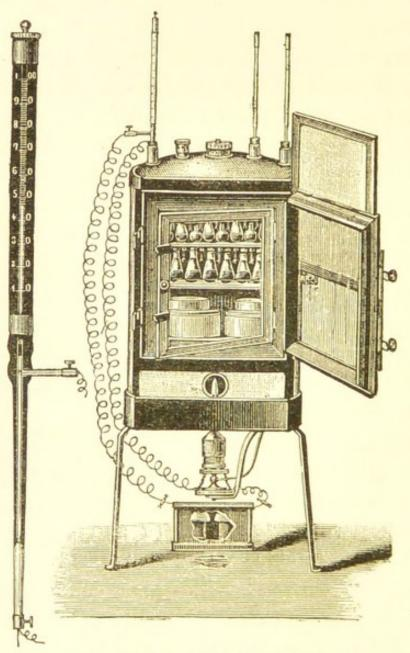
Fig. 16. Karl Abel's Incubator. (With thermo-electric regulator.)
