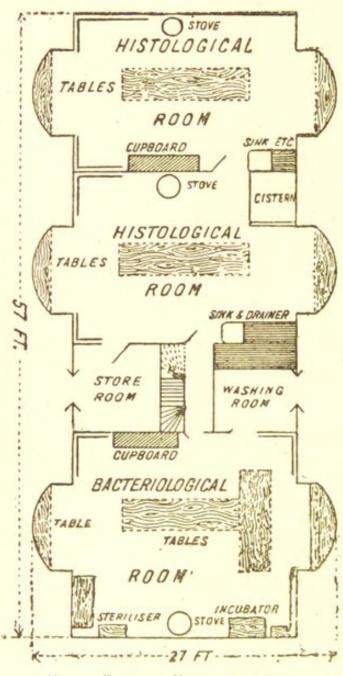
Fig. 1. Plan of Bacteriological Laboratory, etc.
