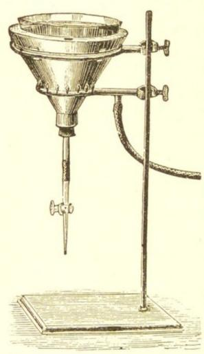
FIG. 19. HOT-WATER FILTER.
