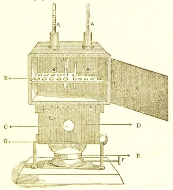
Fig. 11. Hot-air Steriliser heated by Paraffin Oil or Gas. (Devised by Mrs. A. B. Griffiths.)
