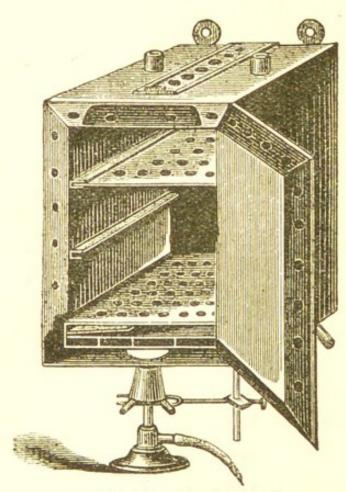
FIG. 10. HOT-AIR STERILISER.
