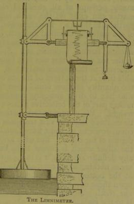
of Limnimeter. The apparatus consists of a *swimmer*, which can be raised and lowered; and by this movement the triangle is turned towards the left,
