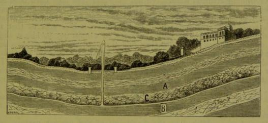
SECTION DRAWING OF ARTESIAN WELL. A B, CLAY STRATA. C, SAND STRATA.
