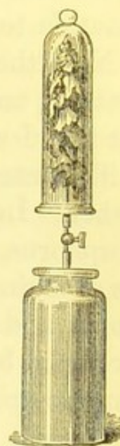
FIG. 28.—Union of Chlorine with Tinsel.
