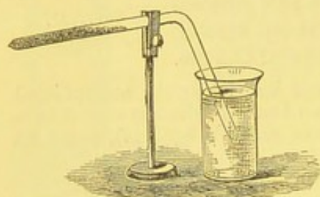
Fig. 145. —Liquefaction of ammonia.
