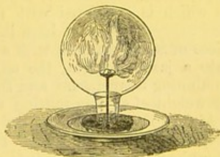
Fig. 25.—Phosphorus burning in oxygen.
