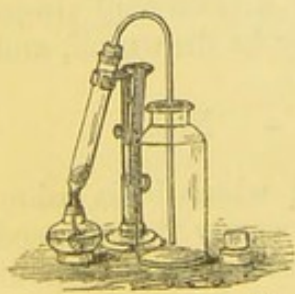
Fig. 163.—Preparation of nitric peroxide.
