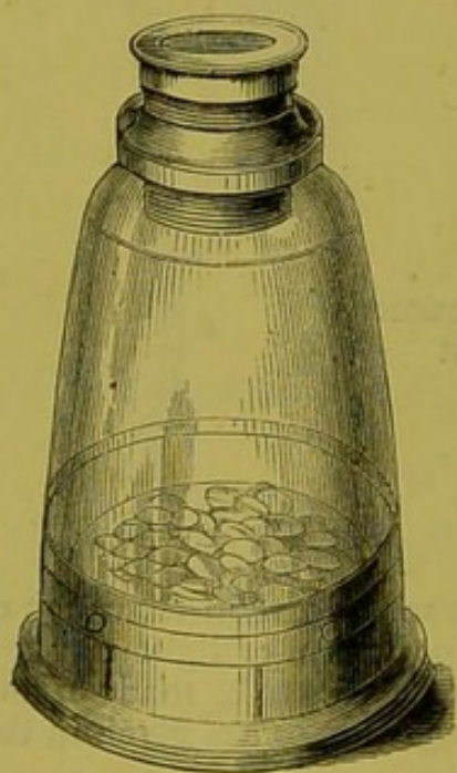
Fig. 65.— Simple Microscope , in which the Lens is focused by turning the Screw.
