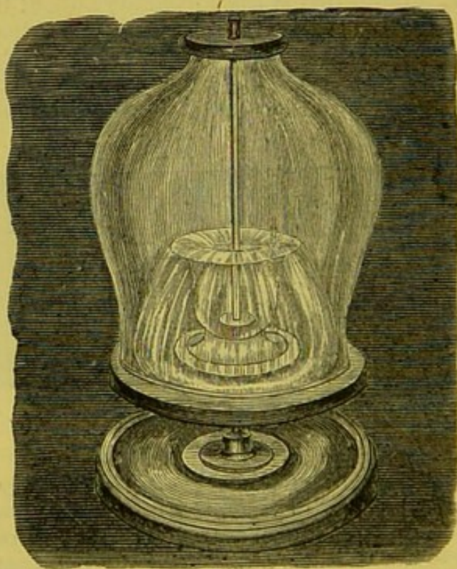
FIG. 365.— Gassiot's Cascade, The current passing into and out of a glass vessel placed in a vacuum.
