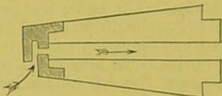
FIG. 257.— Section of the Jet used for the Hydro-Electric Machine, Being a conical plug of hard wood (partridge-wood is preferred), terminated by a brass mouth-piece. The shaded parts are brass.
