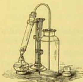
Fig. 146.—Preparation of nitric peroxide.
