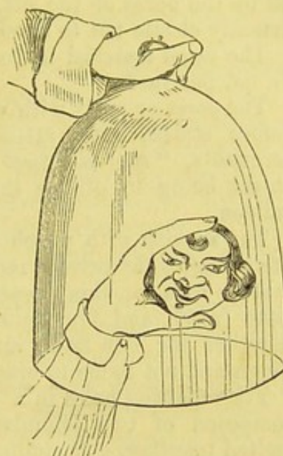
Fig. 114. The squeaking toy, used in a jar of hydrogen.
