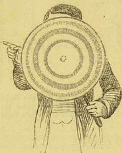
Fig. 304. Design for the phenakistiscope. The spectator is supposed to be looking towards a mirror through the slits. It is supported by a handle through the centre, round which it is twirled by the other hand.
