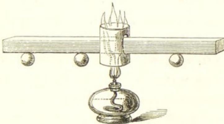
(this is one way of obtaining the power of heat) and place it under that little chimney, the flame will strike against the bar of copper and keep it
