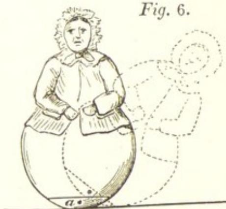
fectly sure, without looking inside the figure, that there is some arrangement by which the centre of gravity is at the lowest point when the image is standing upright; and we may be certain when I am tilting it over (see *fig. 6*) that I am lifting up the centre of gravity (*a*), and
