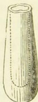
Here is another form of the same kind of experiment. I have here some more glass which has not been annealed [showing some thick glass vessels <sup>(11)</sup> (*fig. 14*)], and if I take one of these glass vessels and drop a piece of pounded glass into it (or I will take some of these small pieces of rock crystal—they have the advantage of being harder than glass) and
