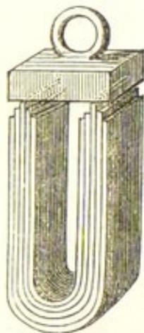
together in order to increase the attraction. This mass will lift that lump of iron, and what is more, by placing this *keeper*, as it is called,
