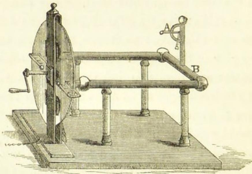
machine arranged for the purpose of rubbing glass with silk, and for obtaining the power called *electricity*; and the moment the handle
