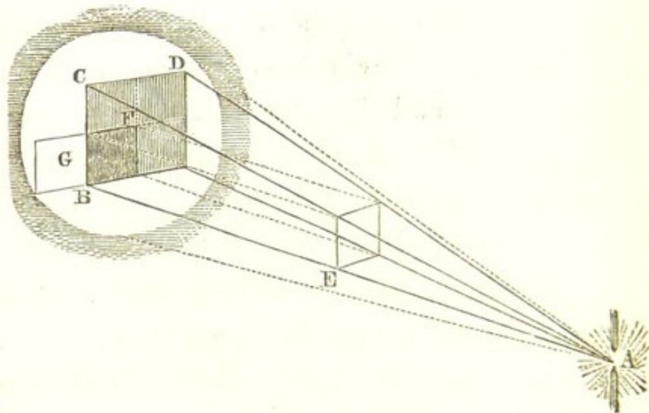
other one in size, and place it midway between the lamp and the screen; now look at the size of the shadow  $B D$ , it is four times the original size. Here, then, comes the “inverse square of the distance.” This distance,  $A E$ , is *one*, and that distance,  $A B$ , is *two*; but that size  $E$  being *one*, this size  $B D$  of shadow is *four* instead of
