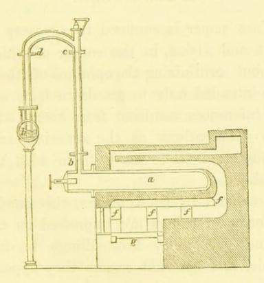
a is the retort; g the grate of the furnace; ff the flues; b c d the dip-pipe; h the condensing main.
