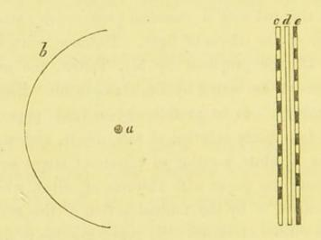
The lime-ball light at a, with a reflector b, admits of this process being conducted easily with artificial light; c represents paper with a series of lines, d the interposed glass, e the photogenic paper, presenting, after having been acted upon, the reverse of the pattern.
