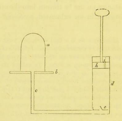
a is the receiver; b is the brass plate, which is generally circular; c is the tube connecting the cylinder with the brass plate; d is the cylinder; e is the valve in the cylinder; h is the piston; i is the valve in the piston.
