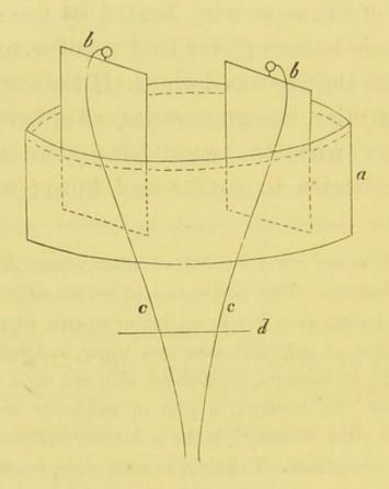
a is the vessel containing the liquid mixture, bb are the two plates, one of copper, the other of zinc, cc are the two conducting wires attached to the plates, d is a connecting wire, and the dotted lines represent the liquid mixture and the plates dipped in it.
