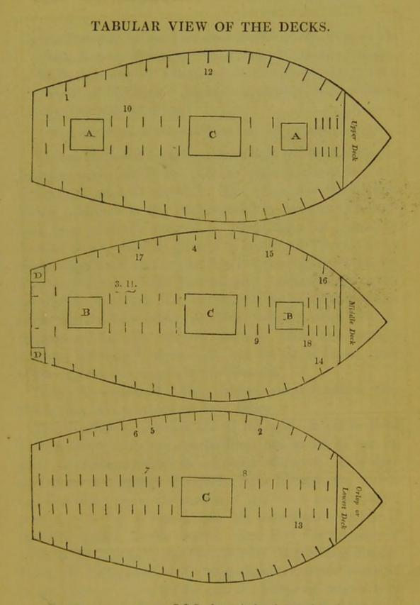
A A, B B, the gangways: C C C, the main hatchway, the only entrance into the hold from the orlop deck: D D, two cabins for female nurses. The short lines represent the fourfold row of beds in the several decks;
