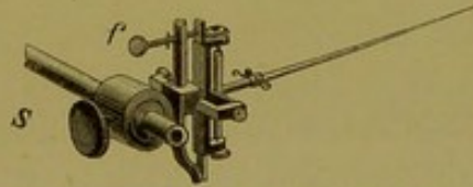
Fig. 1a.—Minute construction of the Recording-lever S with movable screw f .
