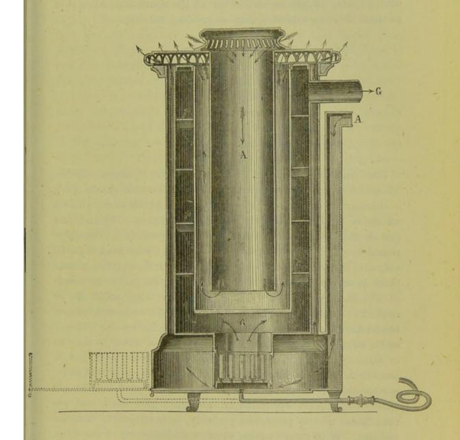
by a pipe at the back of the stove, the opening into the pipe being marked A, and passing down to the air chamber at the base of the stove, gives off a small supply to the furnace chamber for combustion. The main stream is seen to pass upwards between the outer duplicate casings and to be discharged at the top. A second supply enters at the summit of the stove, and following the course
