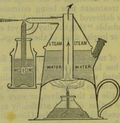
may reasonably be desired. This arrangement of the water inlet, steam chamber, and steam outlet, prevents a very annoying and even dangerous accident of frequent occurrence in instruments with the ordinary form of boiler namely, the forcible projection of spirts
