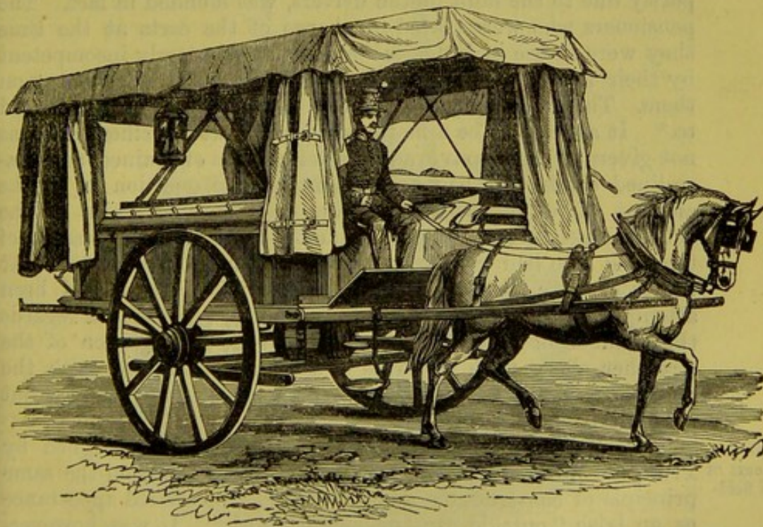
Fig. CXVII.—Guthrie's flat-topped Hospital Conveyance Cart. For carrying two patients lying on spring stretchers on the floor, and a third, if required, in a stretcher slung from the roof, with room also for nine persons sitting on seats before and behind. The second horse is not shown in the drawing.
