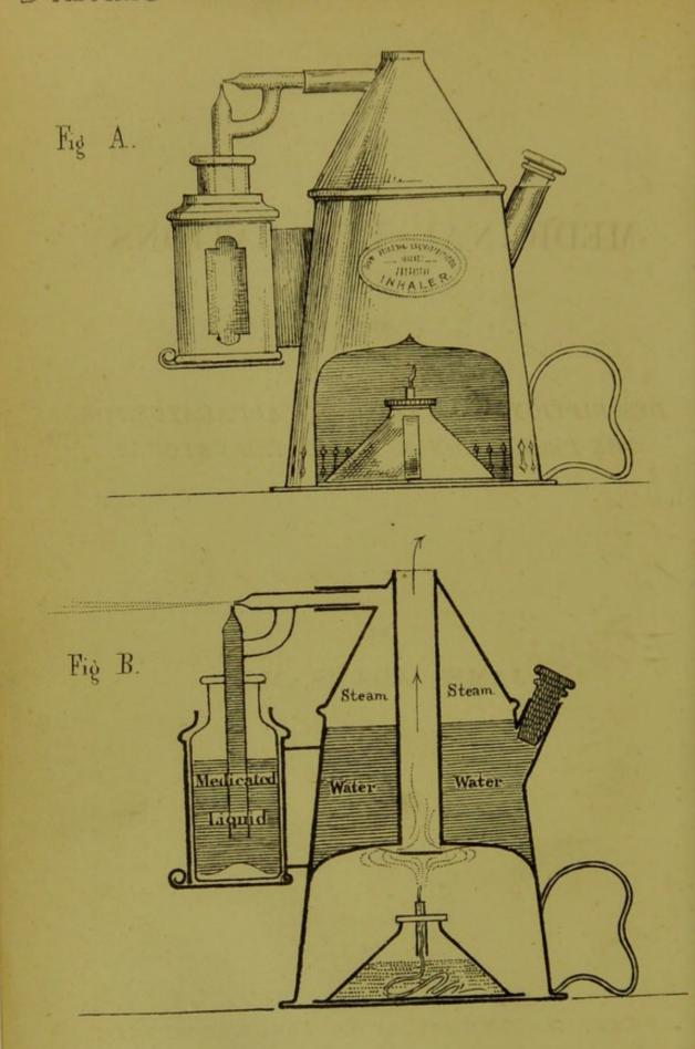
Apparatus for the production of Medicated Vapours. Fig A, External appearance. Fig B, Sectional view.
