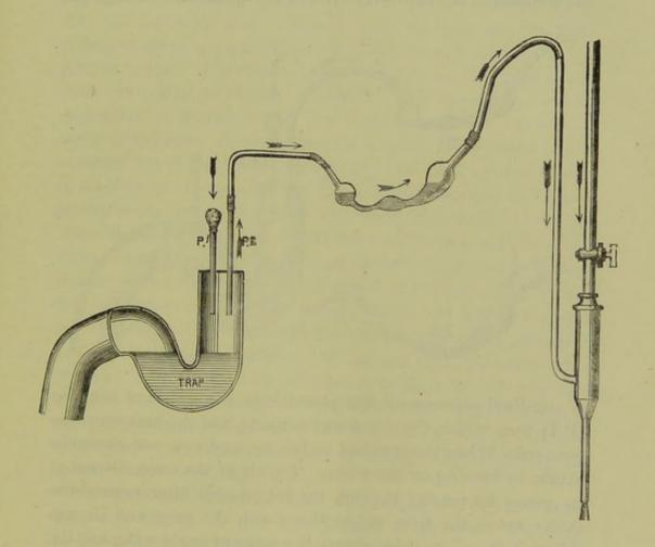
connected with the soil-pipe, and closed on the house by a plate of zinc having two pipes passing through it into the cavity above the water, was connected by one of the pipes (P 2) with a nitrogen bulb—that is, a glass tube—with alternate contractions and expansions. In this bulb was placed a
