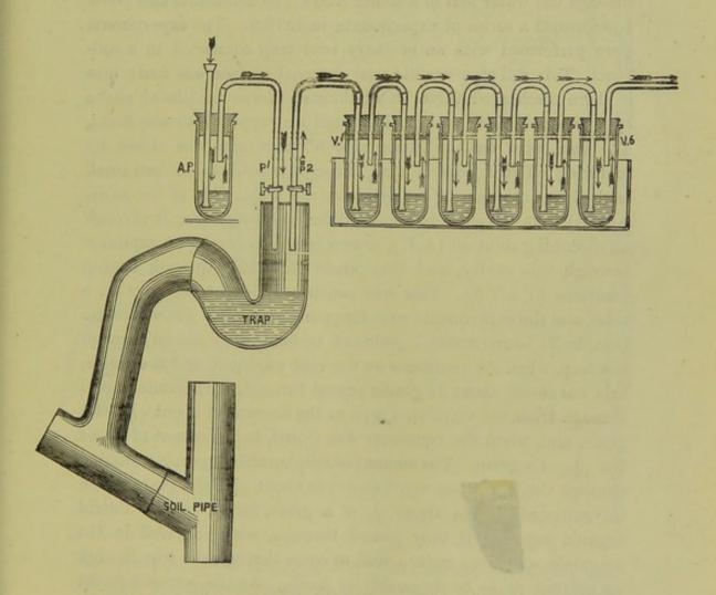
so infinitesimal as to be absolutely harmless. Do the gases pass through the seal of the water trap? The late Dr. Andrew Fergus of this city performed some very interesting experiments with
