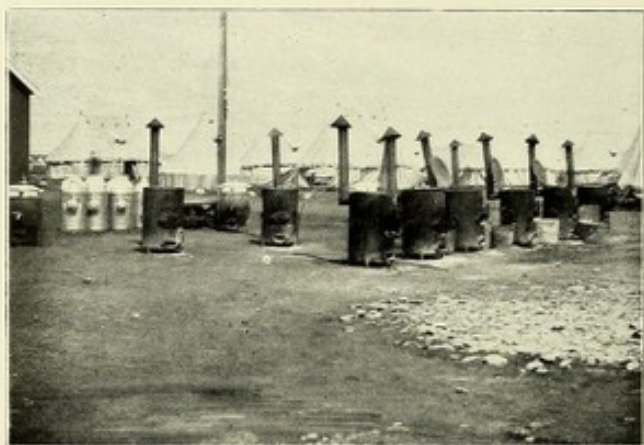
SOYER'S STOVES FOR BOILING DRINKING WATER, AND AYMARD'S STERILISERS NO. 20 GENERAL HOSPITAL.
