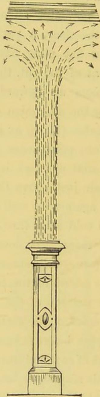
FIG. 8.—Vertical Tube Ventilator.
