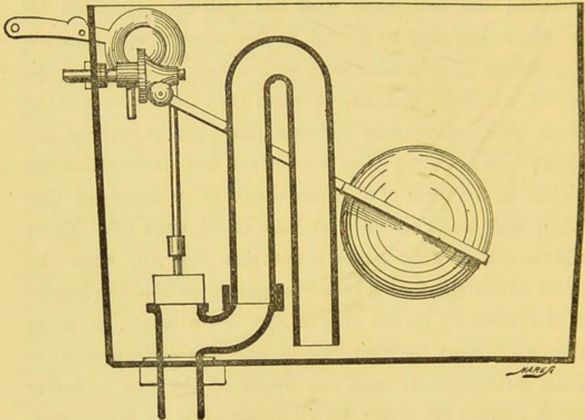
FIG. 42.—Siphon-action water-waste-preventer.
