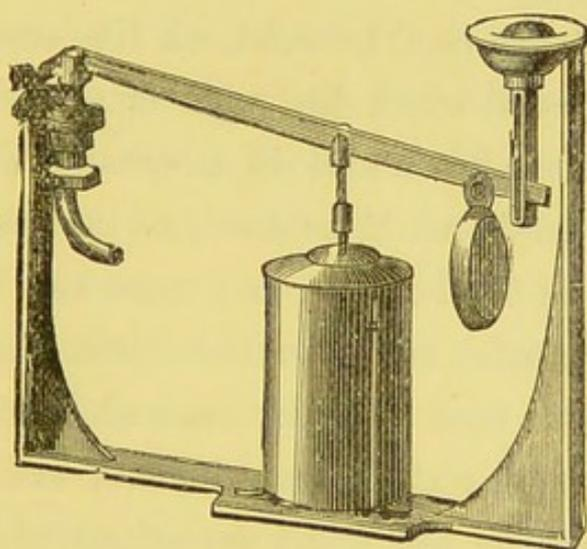
FIG. 43.—Water closet Supply Valve with Bellows Regulator.
