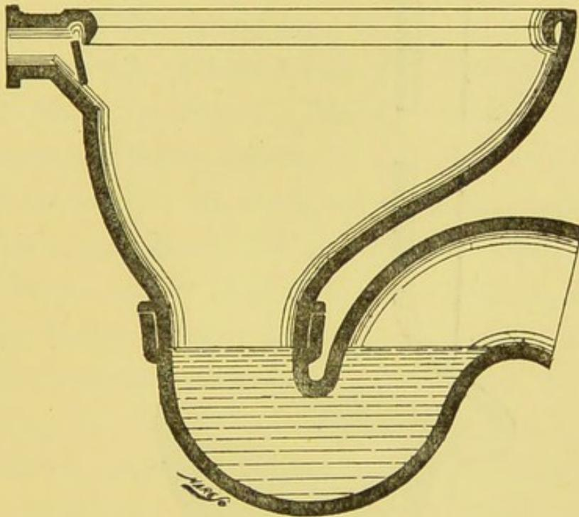
FIG. 34.—Short hopper water-closet with P-trap.
