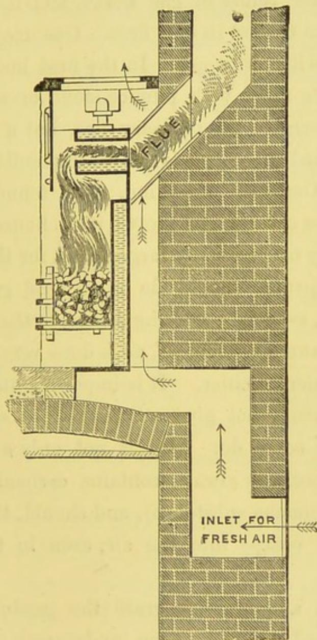
FIG. 17.—Thermohydric Grate (Section).
