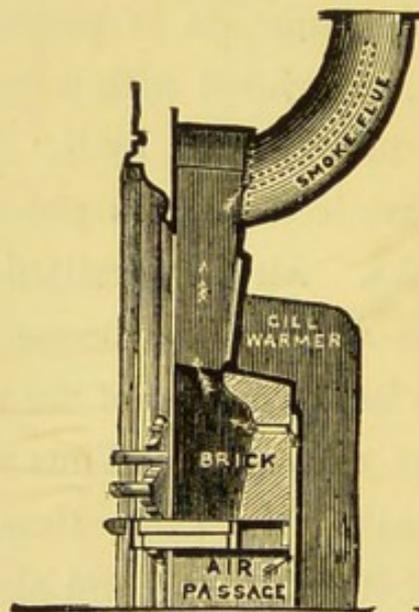
FIG. 14.—The Galton Ventilating Grate.
