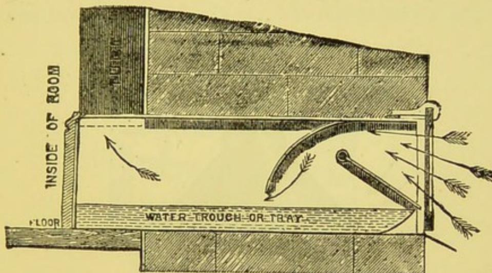
FIG. 9.—Water Tray for Vertical Tube Ventilator.
