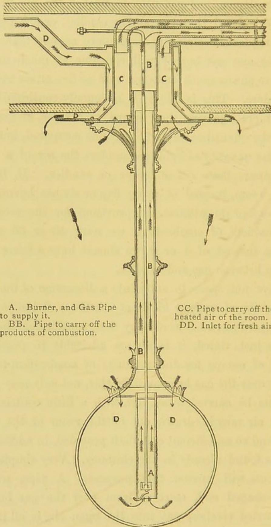
FIG. 13.—Ventilating Globe Light.
