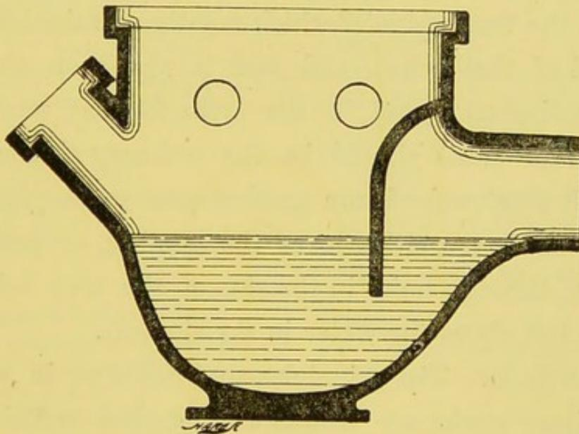
FIG. 45.—Flushing gully.
