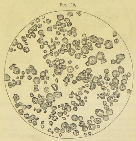
Starch granules of Manihot utilissima, or Tapioca. Magnified 225 diameters.
