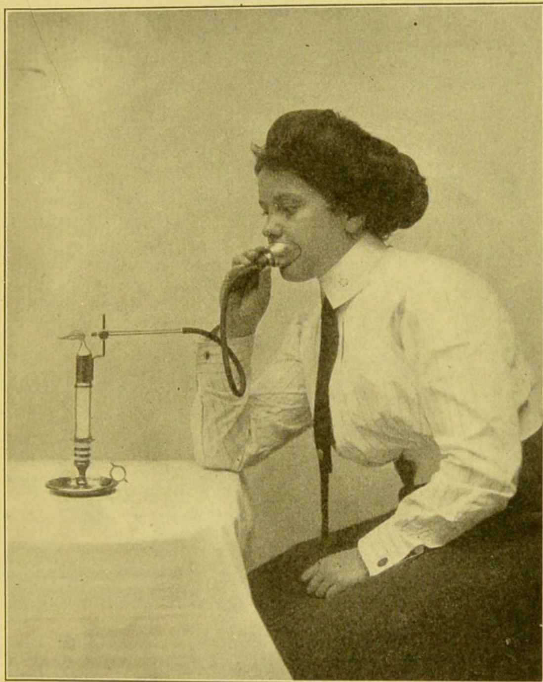
FIG. 42. — Candle flame indicator used for the mouth.
