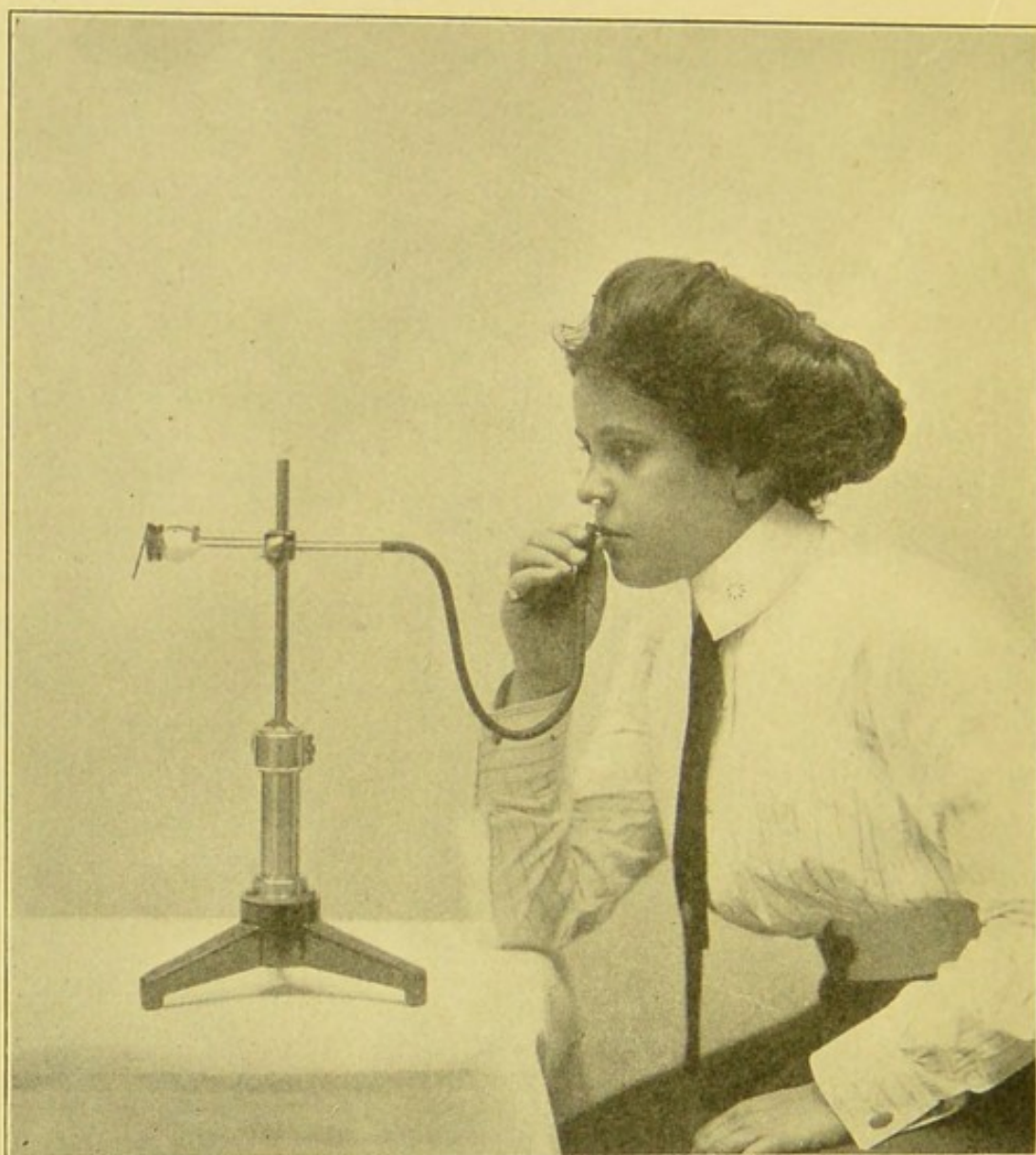
FIG. 43. — Tambour indicator used for the nose.
