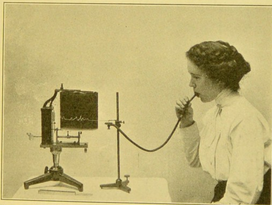
FIG. 3. —Recording the pressure of the lips by the graphic method.
