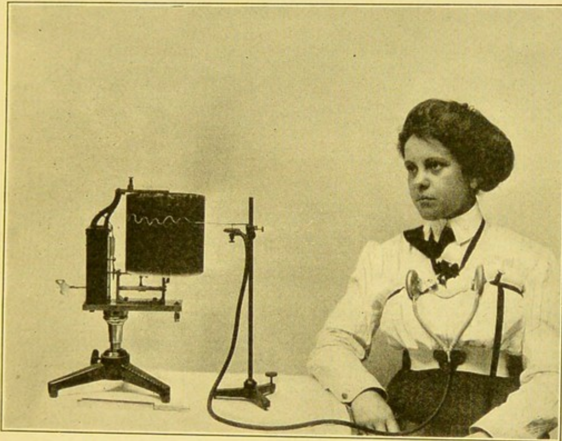
FIG. 1. — Recording the movements of breathing by the graphic method.
