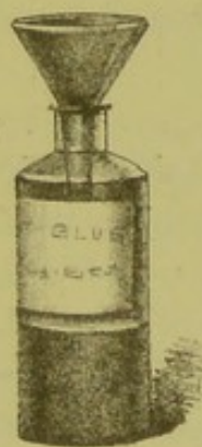
FIG. 12.—Small narrow-mouthed bottle fitted with funnel filter, used especially for aniline staining fluids and aniline water.
