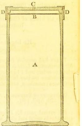
place by the bronzed metallic ring D, which slips over it, and fits the outside of the mouth of the Jar. C, being transparent, both allows light to enter the Jar vertically, and permits the preparation to be inspected from above.
