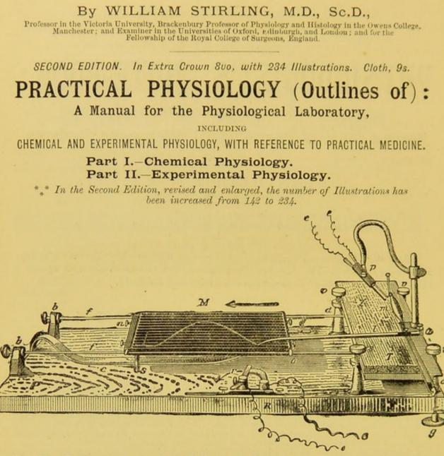
Fig. 118.—Horizontal Myograph of Frédéricq. M, Glass plate, moving on the guides f, f; l, Lever; m, Muscle; p, e, e, Electrodes; T, Cork plate; α, Counterpoise to lever; R, Key in primary circuit.
