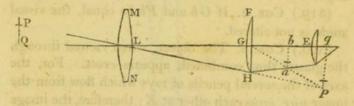
tend to form the image qp, after refraction at the glass FH, form the image ab, between G and q (Art. 223); and this image is viewed through the eye glass E, whose focal length is  $bE^*$ .
