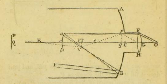
smaller, whose axes are coincident, and whose concave surfaces are turned towards each other; E and e, their centers; T, t, their principal foci, of which, T lies between e and t. In the middle of the larger reflector is an opening, nearly of the same dimensions with the aperture of the smaller, to admit a moveable tube containing a convex eye glass FGH.
