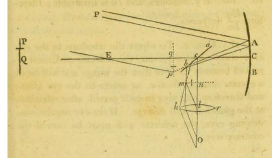
seen through the glass klr, under an angle which is equal to mln; and QP is seen, with the naked eye placed at E, under an angle which is equal to qEp; and since these angles have equal subtenses nm, and qp, they are to each other inversely as the radii ln, qE; therefore the angle which the object subtends at the center of the eye, when viewed with the telescope: the angle which it subtends at the naked eye:: Eq:ln.
