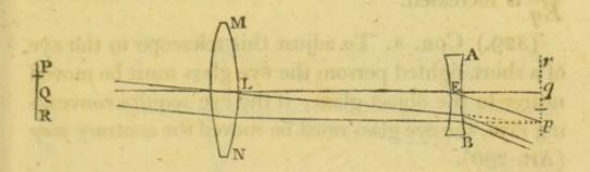
is directed; pqr it's image in the principal focus of the glass L, and therefore in the principal focus of the glass E; then, since the rays tend to form an image in the principal focus of the concave lens E, after refraction at that lens, they will be proper for vision (Art. 290); or, a distinct image of the object PQR, will be formed upon the retina of a common eye.
