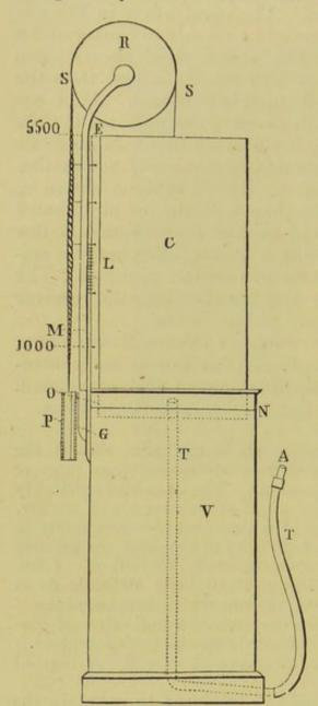
Fig. 80. - Schnepf's Spirometer.\*
