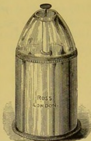
Fig. 144.—Wenham's Parabolic Reflector.
