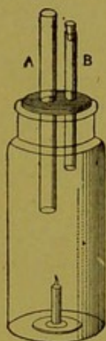
FIG. 129.— Showing the neces- sity of two currents to sustain combustion (Munson.)
