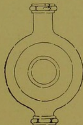
FIG. 152.—Anti-siphon trap. Quartermaster's Department type.
